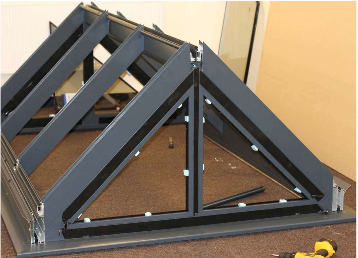
This roof is one of our current jobs (2400mm Projection x 1500mm Width 45 Degree )
